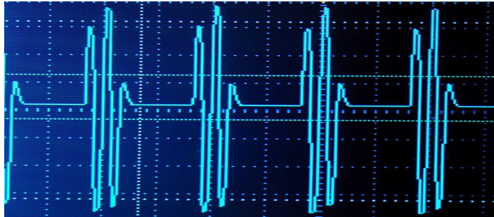
The 909 hz Carrier Occuring @ 40 Hz
